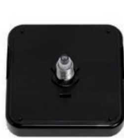
MQCF16NG MOVIMENTO OROLOGIO SENZA GANCIO IN PLASTICA CANOTTO H MM. 16,0 FILETTATURA MM. 10,0 Clock movement 16,0 mm without plastic hanger Total shaft length 16,0 mm / Shaft length to screw 10,0 mm
