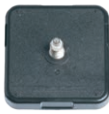
MQCF16SNG MOVIMENTO OROLOGIO SENZA GANCIO IN PLASTICA CANOTTO H MM. 16,0 FILETTATURA MM. 10,0 Clock movement 16,0 mm sweep without hanger Total shaft length 16,0 mm / Shaft length to screw 10,0 mm
