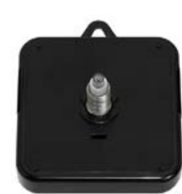
MQCF19 MOVIMENTO OROLOGIO CON GANCIO IN PLASTICA CANOTTO H MM. 19,0 FILETTATURA MM. 13,0 Clock movement 19,0 mm with plastic hanger Total shaft length 19,0 mm / Shaft length to screw 13,0 mm
