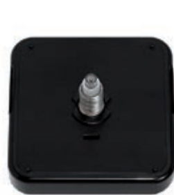
MQCF19NG MOVIMENTO OROLOGIO SENZA GANCIO IN PLASTICA CANOTTO H MM. 19,0 FILETTATURA MM. 13,0 Clock movement 19,0 mm without plastic hanger Total shaft length 19,0 mm / Shaft length to screw 13,0 mm
